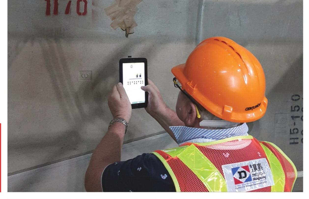
At Hong Kong's Liantang Lung Shan highway tunnels, strain gauge modules were embedded inside concrete. The information relayed back to a data logger that was accessible by Bluetooth
